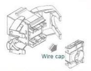
Ensure the wired cap follows relative position as the latch, and cover it with both jaws.
