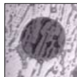
Left: Fingerprint oils on a connector end-face. Right: A properly cleaned connector end-face
