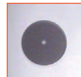
Below: A properly cleaned connector end-face
