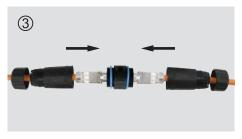
3. Insert the patch cords into the both ends of the RJ45 coupler.
